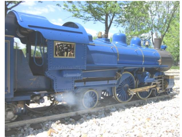
1 1/2" scale 4-4-2 Atlantic Coal-fired Steam Locomotive
