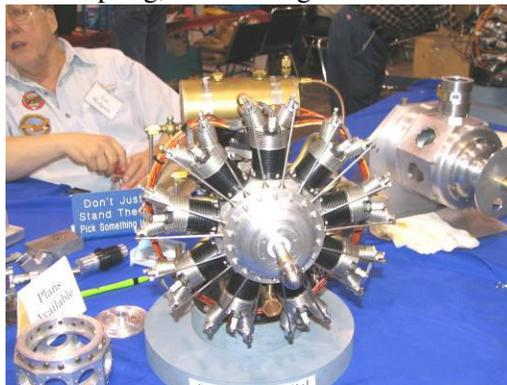
**Nine-Cylinder Radial Aircraft Engine**
